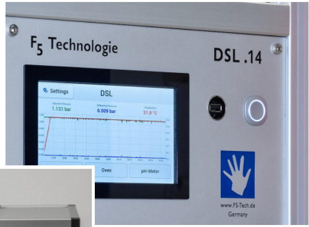
PLC with colour touch screen and big data display
