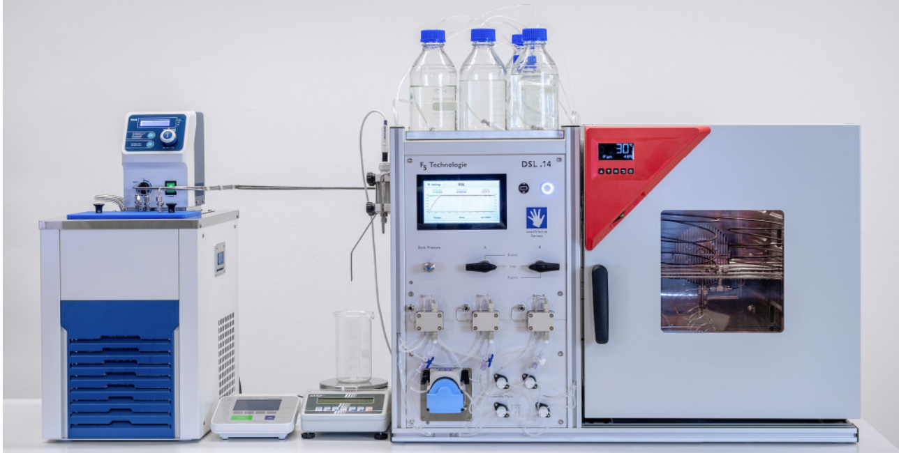
Cooling options: by liquid bath or by cooled air inside the oven
