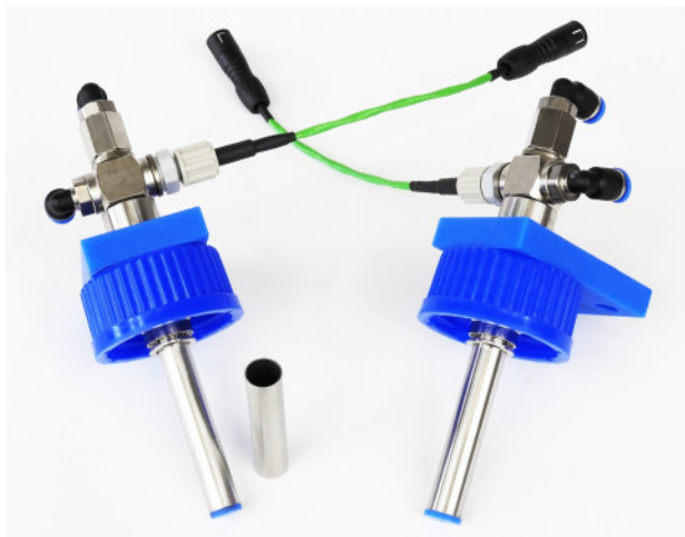
Cold finger unit with insert with removable sleeve (left) and with standard insert (right)
